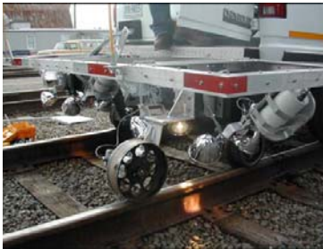
A hairline fracture (above) that can be detected by the FRA Automated Optical Track Joint Bar Inspection System (below).
