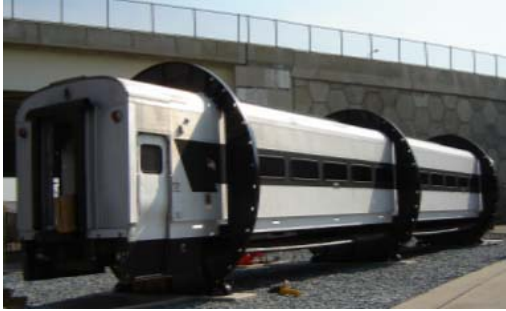
The Passenger Rail Vehicle Emergency Evacuation Simulator or “Rollover Rig.”
