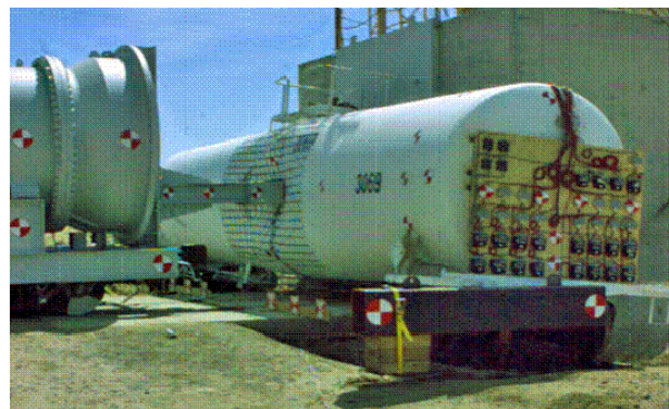
One of a series of crash impact tests performed in the development of the FRA / PHMSA proposed rule to strengthen rail hazmat tank cars.
