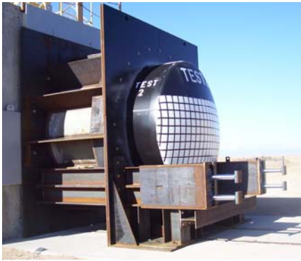
A head-end shield developed for use in a crash impact test for the Next Generation Rail Tank Car project.
